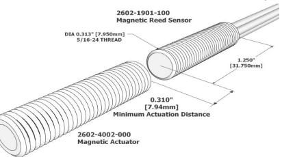
All measurements are in Inches [millimeters]
