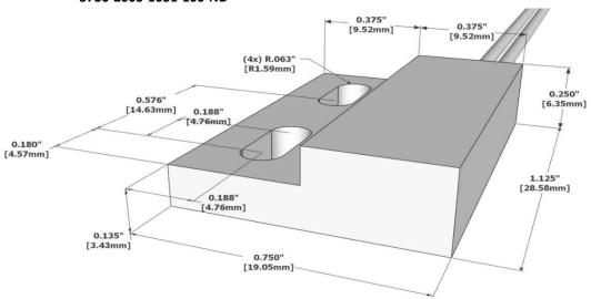
All measurements are in Inches [millimeters]
